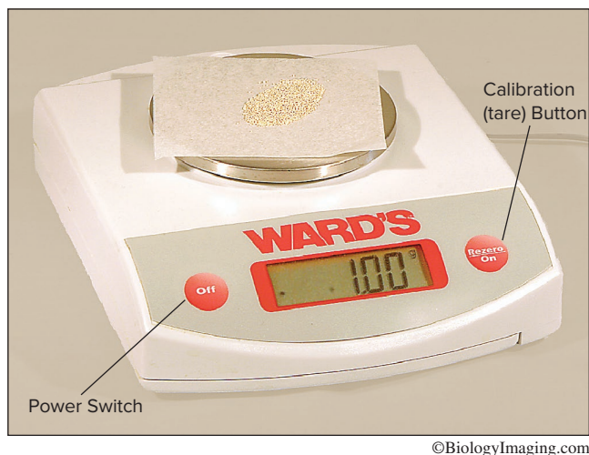
Figure 2.4 Biologists use balances to measure mass. (A) The parts of a triple-beam balance include the (a) zero-adjustment knob, (b) measuring pan, (c) movable masses on horizontal beams, and (d) balance marks. (B) A top-loading balance has a measuring pan, a power switch, and a zero calibration (“tare”) button.
