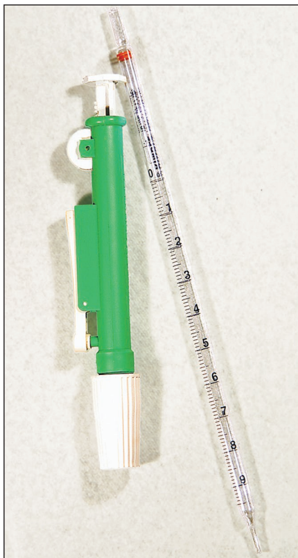
Figure 2.2 A pipet is used to extract and dispense volumes of liquid. A suction device (shown in green on the left) draws fluid into the pipet, and graduated markings on the pipet allow precise measurement of a fluid's volume. Never use your mouth to suck fluid into a pipet.
